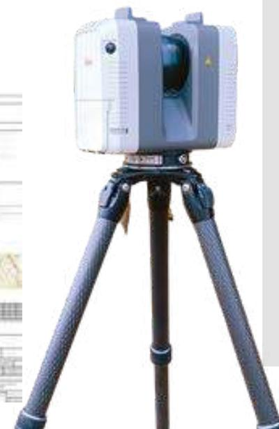
Scanner terrestre LiDAR
